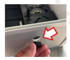
2. Remove the HVAC JUMPER plug and connect the HVAC SENSOR CABLE as shown.
