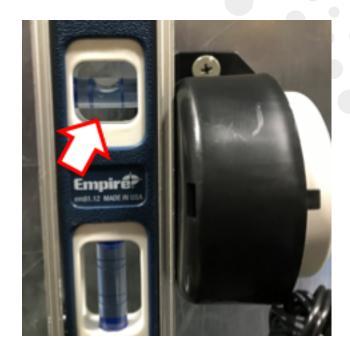
11. DO NOT OVER TIGHTEN THE SET SCREW IN THIS STEP, AS IT WILL DAMAGE THE SENSOR! While maintaining the vertical position, GENTLY HAND TIGHTEN the set screw just enough to hold the sensor in the desired position. The set screw compresses the adapter tube — this compression holds the sensor in place.
