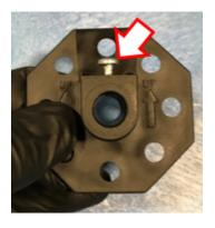
4. Insert the Aluminum tube into the center hole of the injector mount as shown. Using a tape measure, set the length to reach to the center of the duct, or leave at least 1" of tube exposed as shown. Gently tighten the set screw as needed to positively maintain the position of the Aluminum tube:
