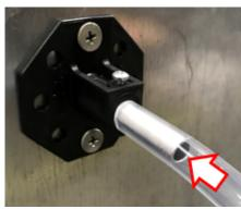
13. Secure the tube with a zip tie at the midpoint of the Aluminum tube. Tighten the zip tie as needed to secure the tubing in place, and cut off the excess zip tie to complete the injector installation.
