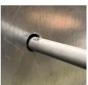
3. <u>Start</u> the set screw into the injector mount as shown. Do not allow the screw to poke through into the center at this time:
