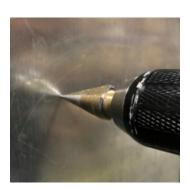
2. While securely holding the Aluminum tube, check the fit to the hole – it should pass freely into the injection port with a minimum gap:
