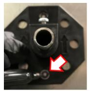
9. Remove the injection assembly and pilot drill the marked mounting holes with a 1/8" diameter drill:
