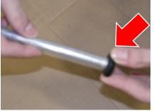
8. Connect tubing to the air probe
