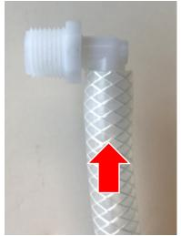
4. Insert the assembly into the access hole in the cabinet ("UP" orientation shown is preferred):
