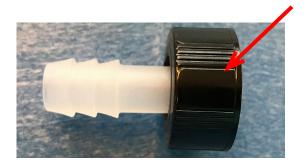
3. Push Injector Tubing (#4) over the barbed portion of the Stem (#1c), allowing a *small gap* between the end of the tube and the Cap (#5) as shown.
