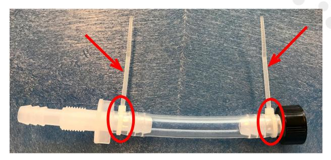
6. Cut off the excess Cable Tie (#3) tails.
