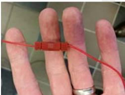
2. Bundle the wires and tube inside of the sleeve.
