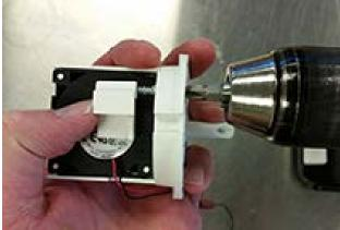
3. Push one end of the tubing onto the fitting on the back side of the base housing part, just below the fan tray, and rotate the clips in toward the fan on both sides.
