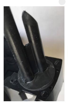
8. Insert the PITOT ASSEMBLY into the 7/8" dia. hole that was drilled into the duct so that the 'FLOW' graphic matches the AIR FLOW DIRECTION. Apply sufficient pressure to the PITOT ASSEMBLY until the SNAPs firmly engage the back side of the duct wall.
