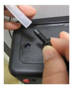
12. Fully insert the NON barbed end of the UNIVERSAL CONNECTOR into the vertical PLUME PORT of the cartridge within the appliance. NOTE: this connection must be reversed to change the cartridge!
