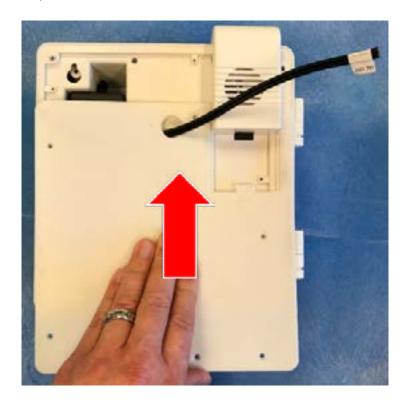
8. Use six screws to secure the panel.
