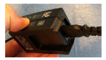
4. Connect power jack into the appliance, wrap excess cord and stuff into cavity.
