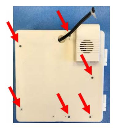
9. The hole in the shroud is sized to fit the smallest standard track light adapter. If your track light adapter has a larger thread you may need to expand this hole.
