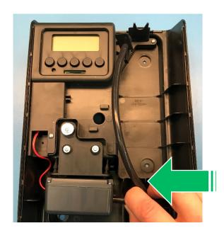
7. Ensure that the short tube is <u>fully engaged</u> with the pump connection, and that the vertical tube is oriented as shown
