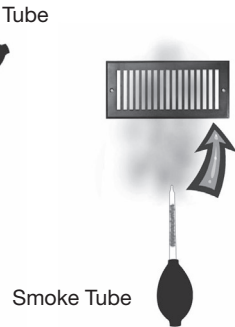
Figure 3 Smoke travels toward grill
