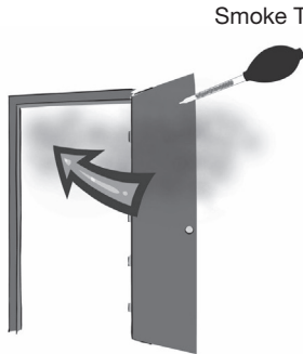
Figure 1 Smoke flows away from door
