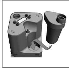
5. To activate cartridge and relieve pressure from shipping: using a tissue or paper towel, press in the stem in the center of the top output chimney; the stem should spring back.
