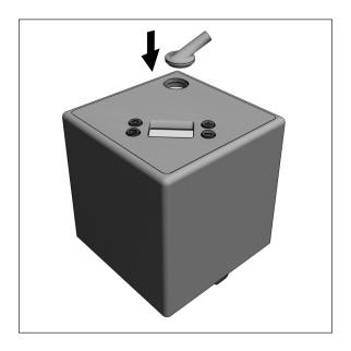
8. Position the AirQ appliance in desired location. AirQ must not be tilted or turned upside down when cartridge is inside; otherwise there will be a spill.
